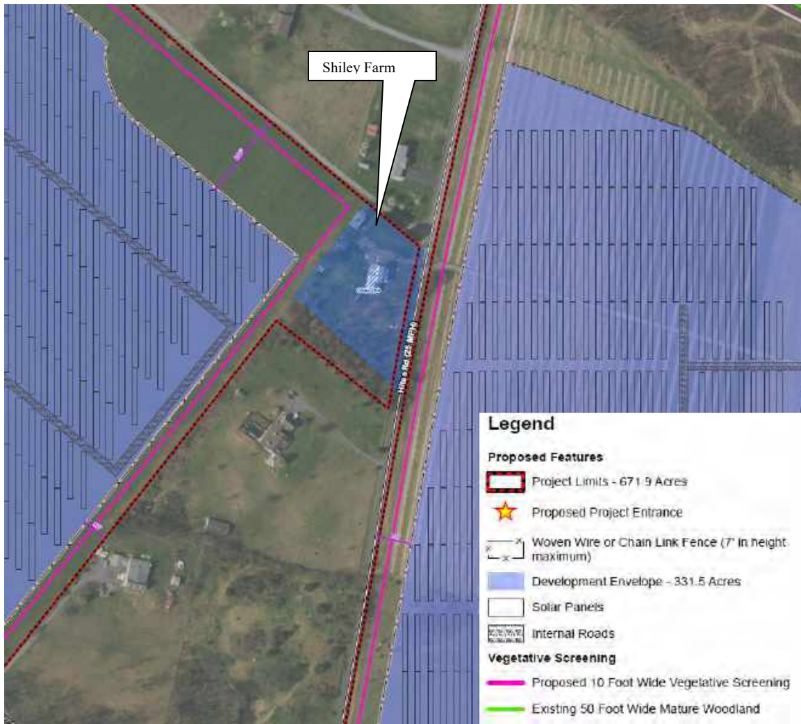
Figure 5: Location of Shiley Farm in relation to the project area showing proposed setback and vegetative screening. Source: Urban Grid
